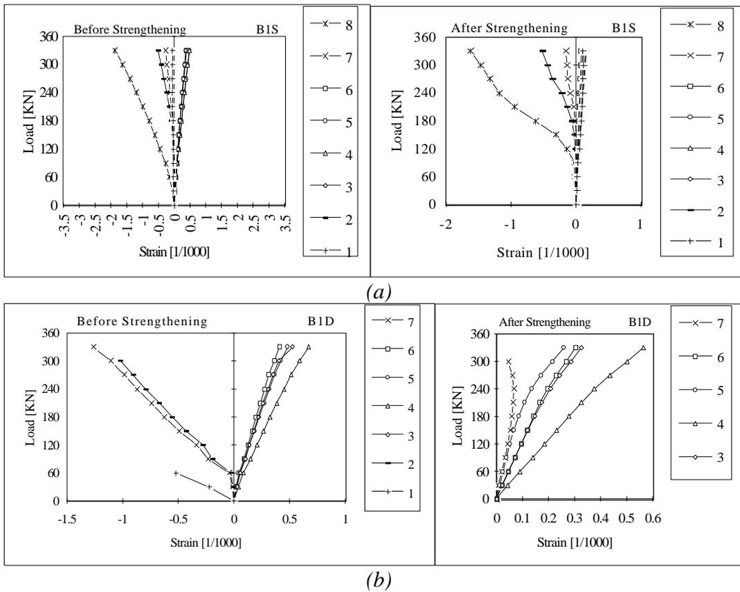
Fig.5 Concrete strain distribution with increasing of the loads at the max. positive moment section of beams in series I
