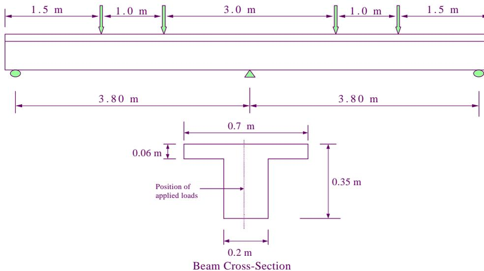
Fig.1 Beams set-up and the load position
