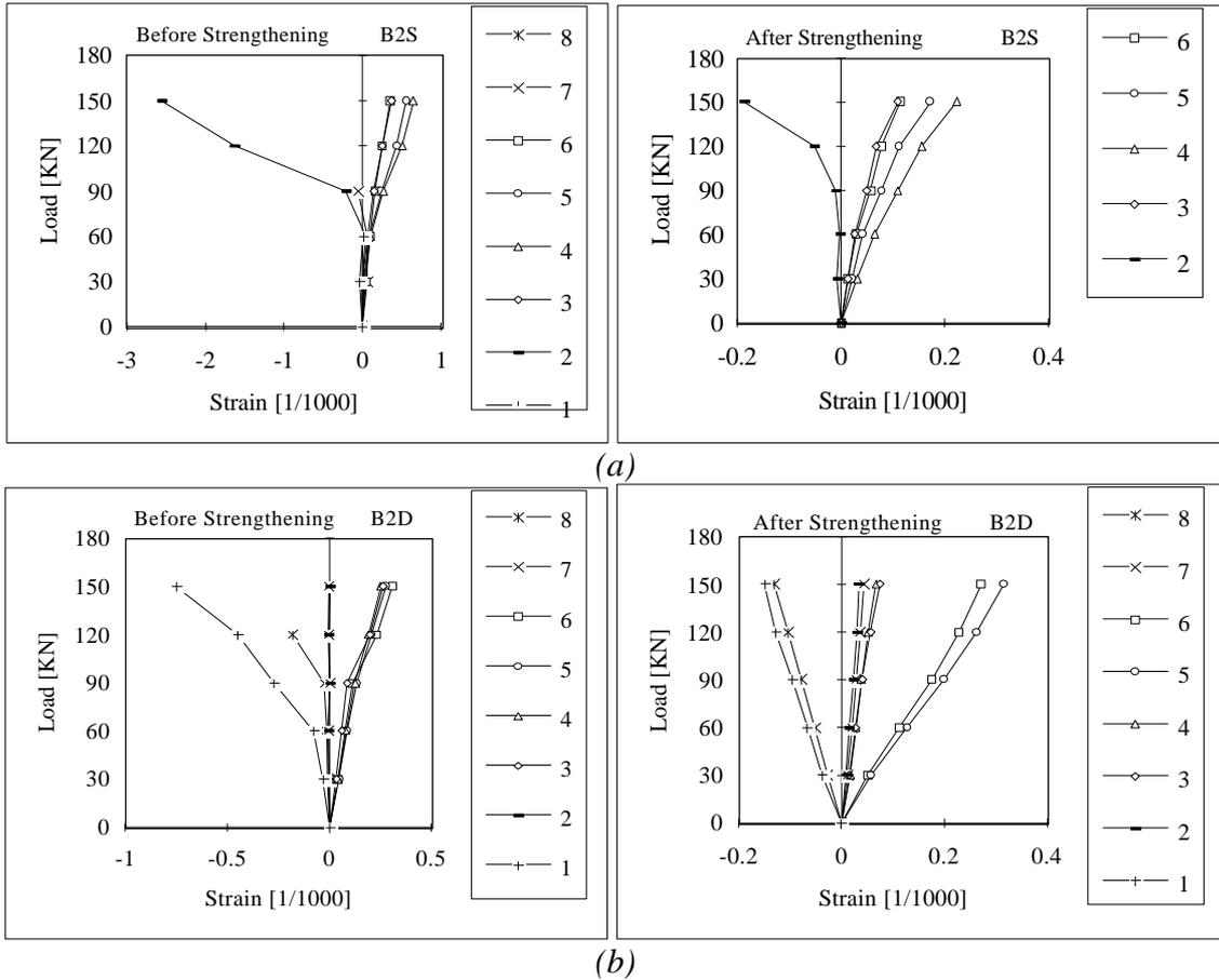
Fig.6 Concrete Strain distribution with increases of Loads at the max. positive moment section of beam in series II
