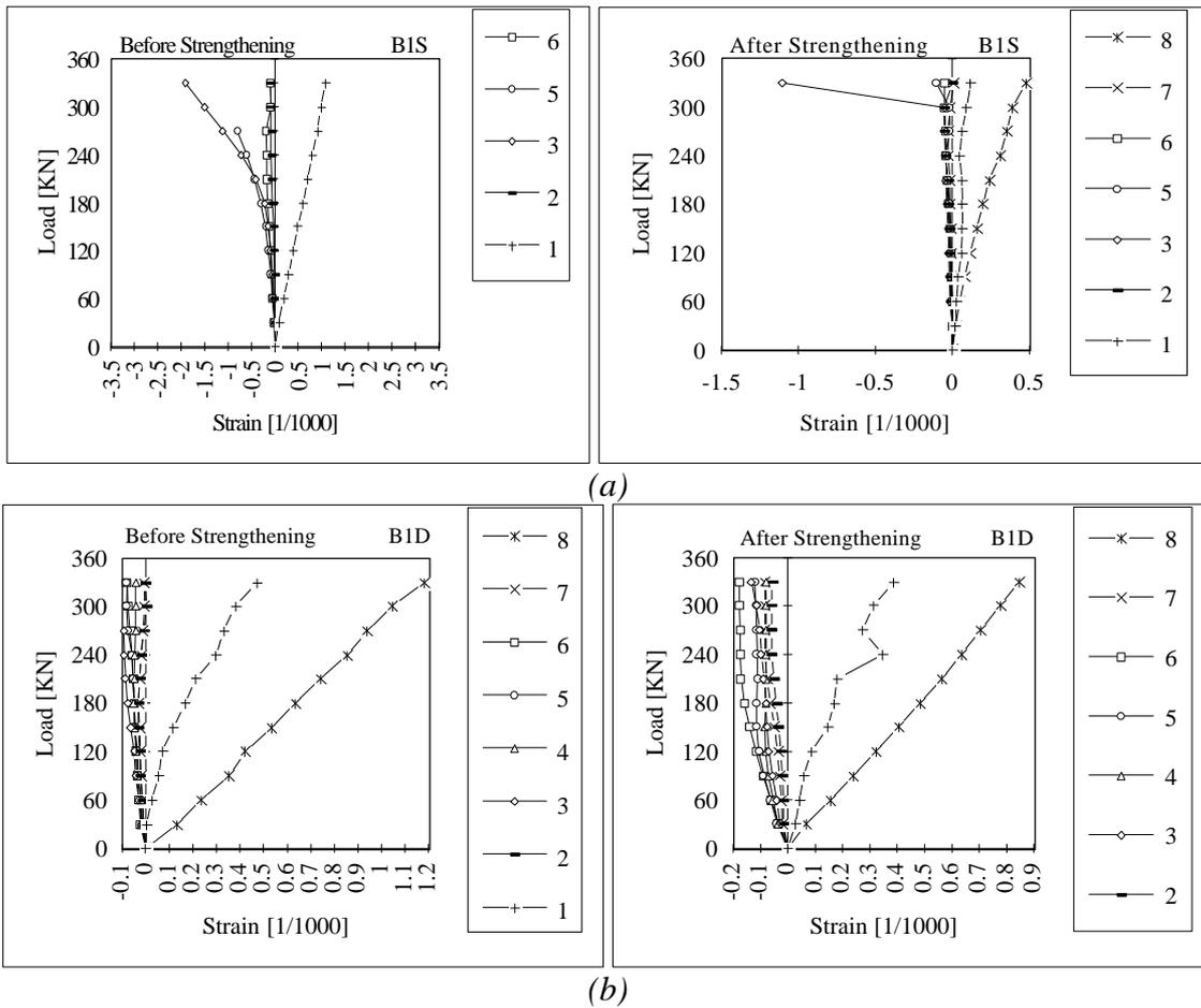
Fig.7 Concrete strain distribution with increasing of the loads at the max. negative moment section of beams in series I
