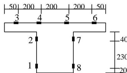
The position of the strain gauges (1- 8) at sec. a-a and sec.b-b (all dimension in mm)
