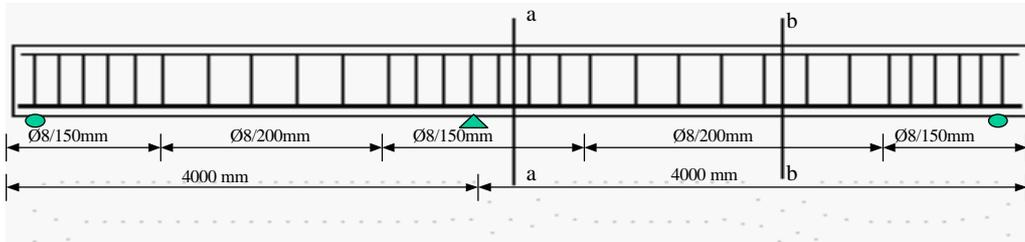
Fig.2 Beam reinforcement arrangement
