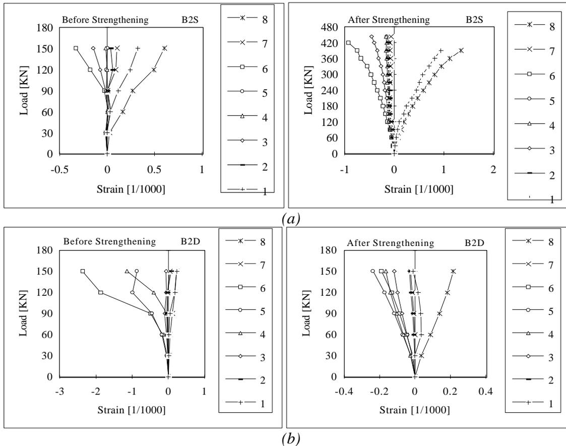
Fig.8 Concrete Strain distribution with increases of Loads at the max. negative moment section of beams series II
