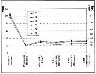
Fig. 4 Changes in the MBN values in the function of time
