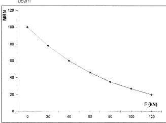
Fig. 3 Calibration curve of the tendon of an UBx type prestressed concrete beam
