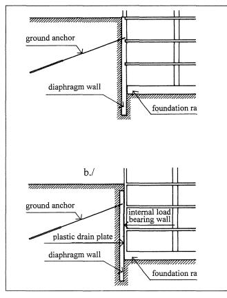
Fig. 1 Connection of diaphragm wall and basement floor slabs.
