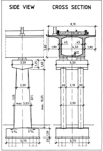
Fig. 5 Structural elements of the viaduct being built
