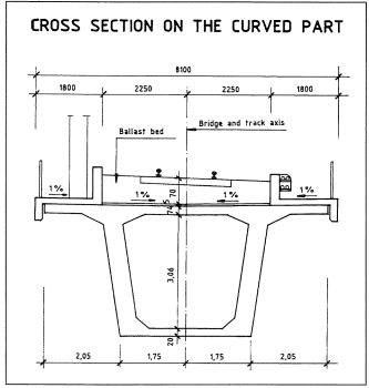
Fig. 2 Transverse section of prestressed concrete bridge elaborated in the tender plan
