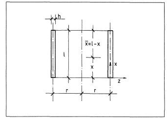
Fig. 2 Geometrical data and coordinate system of analysis
