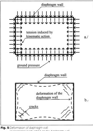
g. 5 Deformation of diaphragm wall (a) horizontal loads acting on the diaphragm wall (b) deformation and cracks of the diaphragm wall
