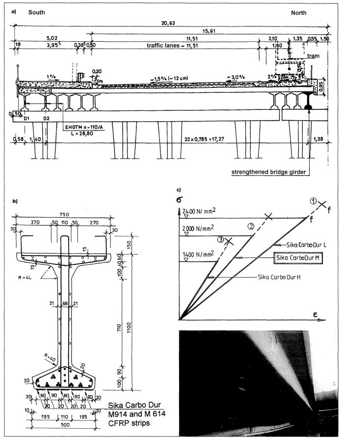
Fig. 7 Strengthening of a prefabricated prestressed pre-tensioned concrete bridge girder in Budapest, Petőfi bridge owing to the failure of some prestressing strands due to corrosion. (Date: Sept. 1997, Strengthening strips: Sika CarboDur H914-56 m and M614-84 m. Designer: Budapest University of Technology: Dr. György L. Balázs and Dr. György Farkas. Exec: Pannon Freyssinet Ltd.) a) Cross-section of the bridge
