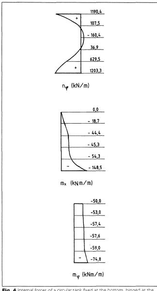
Fig. 4 Internal forces of a circular tank fixed at the bottom, hinged at the top (  $t_i=0~^{\rm o}C,t_{\rm o}=-30~^{\rm o}C)$
