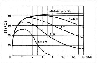
Fig. 4 Increase of the concrete core temperature due to hydration. (300 kg/m<sup>3</sup> Portland cement CEM I 32.5 R)
