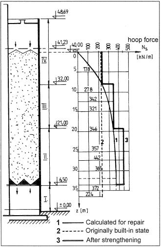
Fig. 5 Limit hoop-forces and ring-forces
