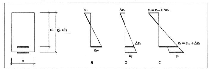
Fig. 9 Stress-strain diagrams before and after strengthening a) Strains before strengthening b) Strains from loads above strengthening c) Strains of strengthened member
