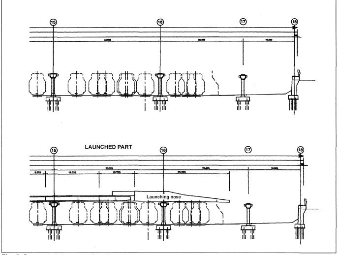
Fig. 6 Construction phases over the railway
