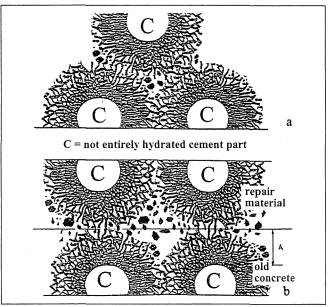
Fig. 2 Sketch of the joint of a silicate frame, a) in a state when they are not completely grown together, b) their principal scheme
