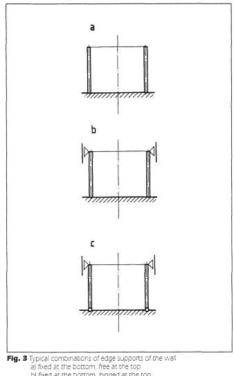
b) fixed at the bottom, hinged at the top c) hinged at the bottom and at the top
