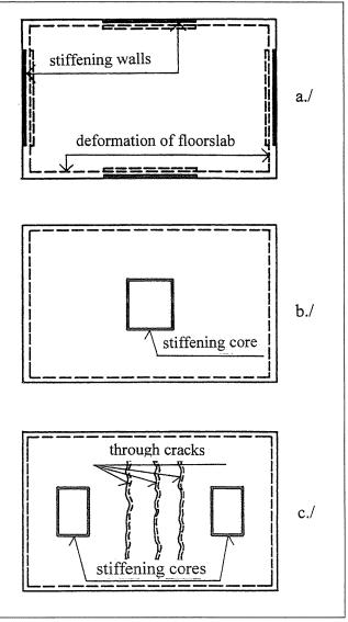
Fig. 6 Effect of the arrangement of stiffening structures: a) favourable
