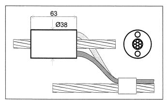
Fig. 1 Sensors pulled onto tendons built-in UBx typr prefabricated, prestressed concrete beams
