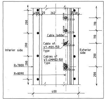
Fig. 4 Reinforcement of cylindrical wall, detail
