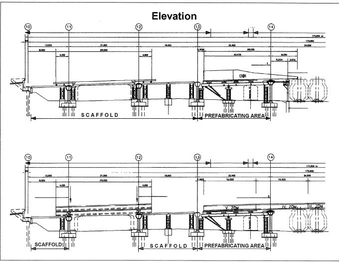
Fig. 5 Structure built on scaffold and the beginning of incremental launching
