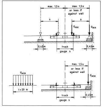
Fig. 3 Examination the effect of a derailed vehicle by EUROCODE
