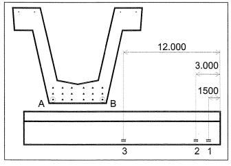
Fig. 2 Arrangement of tendons in an UBx type prestressed concrete beam and the location of sensors
