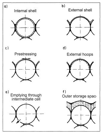
Fig. 4 Methods of strengthening
